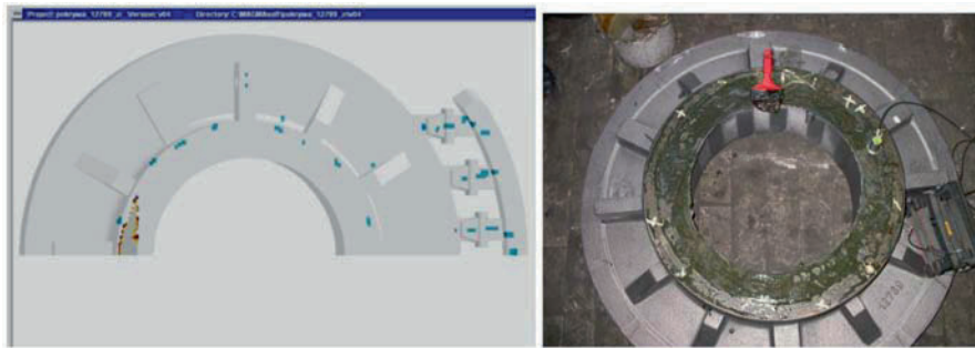
Fig. 7. Comparison of defects location in virtual (from Magmasoft) and real ductile cast iron industrial casting (detection by ultrasonic testing – UT).
