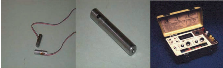
Fig. 3. Pins with strain gages, shaft and P3500 instruments used to measure the strain.
