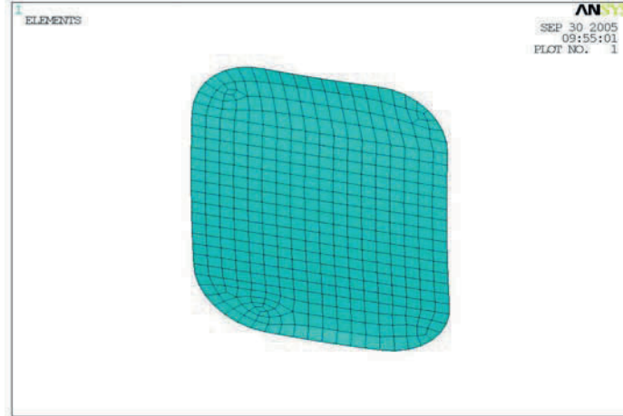
Fig. 6. The shell model of the gap and flush.
