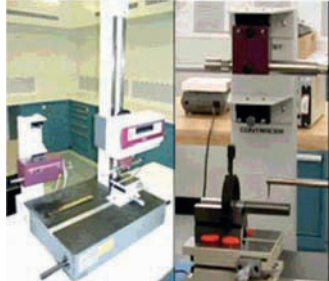
Fig. 5. Profilo-roughometer Mitutoyo SV4000.
