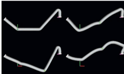
Fig. 5. Manipulation in a virtual environment: example of deformed hose for four load cases.
